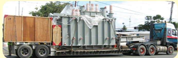
Trailer with 40/50MVA, 66/33kV Transformer arrives at Milford Bay Substation
